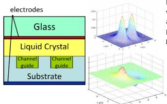
liquid crystal modelling capabilities with wave propagation methods, modal analysis and beam propagation methods. In particular, we are interested in reconfigurable LC photonic structures using
