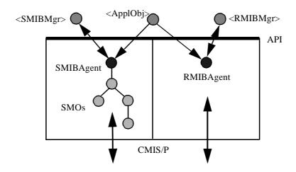
Figure 4 The Remote and Shadow MIB Manager Access Models.
