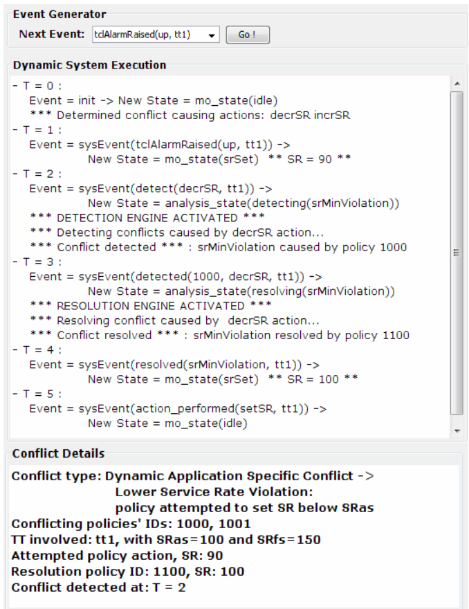
Fig. 10. Analysis example of a dynamic conflict: detection and resolution.
