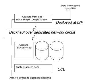
Figure 2: The structure of the  $10\mathrm{Gb/s}$  monitor elements used within the MASTS project.
