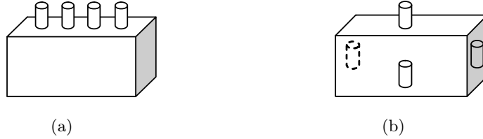
Figure 2: Configurations for the receiving antennas, (a) ULA with equal spacing = \lambda/2 between dipoles, and (b) 3D array arrangement.
