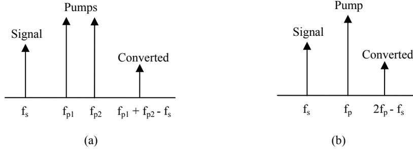
**Figure 1 – (a) Non-degenerate Four-wave Mixing (b) Degenerated Four-Wave Mixing**
