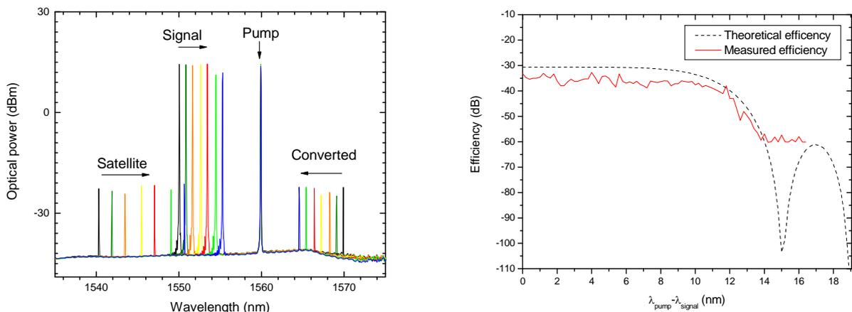
**Figure 3: (a) Measured spectra for different input signals (b) Four-Wave Mixing conversion efficiency**
