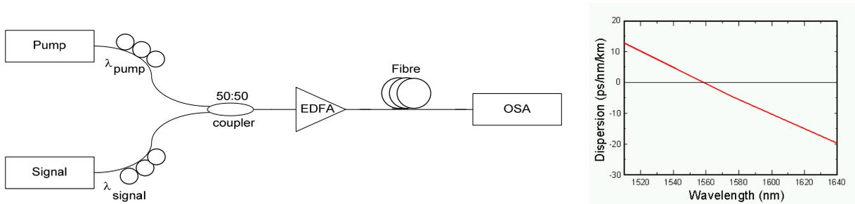
**Figure 2: Experimental setup and chromatic dispersion characteristic of the PCF**
