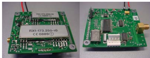
Figure 6. Picture of the PCB hosting the initial platform for developing the radio and network platform for SECOAS. (Picture courtesy of Steve Fitz)
