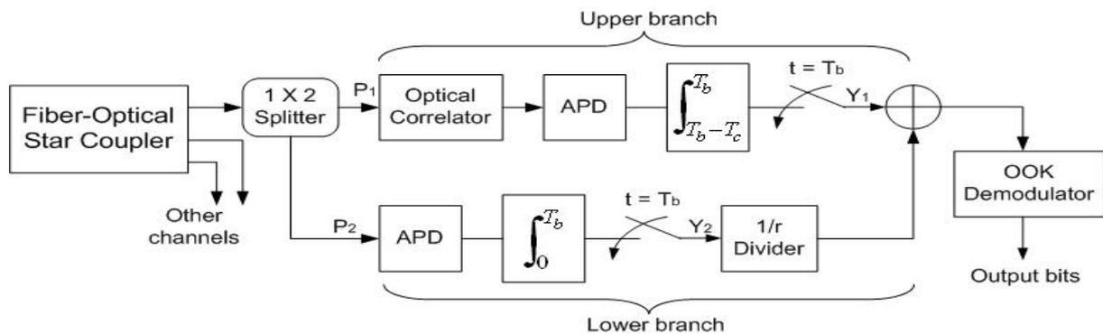
Figure-1: The receiver Structure
