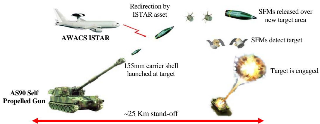
Figure 3 Ballistic SFM dispensed over a target area
