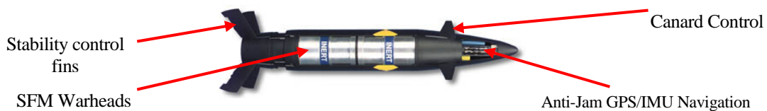
Figure 4 Sectioned view of Excalibur GBS
