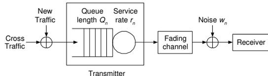
Figure 2: The queueing and wireless channel model for single-hop packet transmissions.
