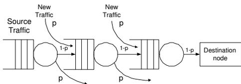
Figure 1: System model for WMNs.
