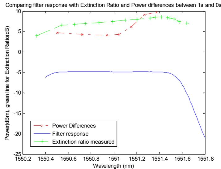
**Figure 6 Comparing filter response with ER and Power differences between energies of the “1s” and “0s”**
