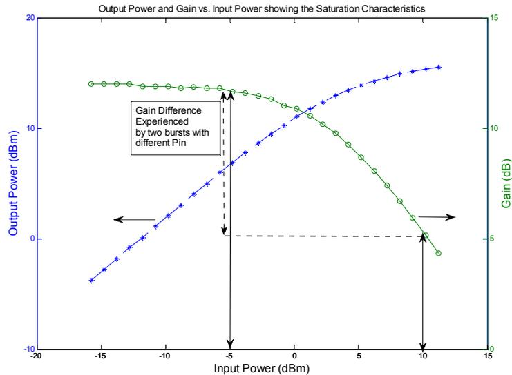
**Figure 2 Output power and Gain vs. Input Power showing the saturation of the Booster SOA**
