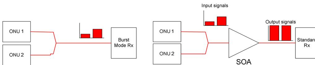
Figure 1 Optical Burst Equalisation allowing standard receiver to be used
