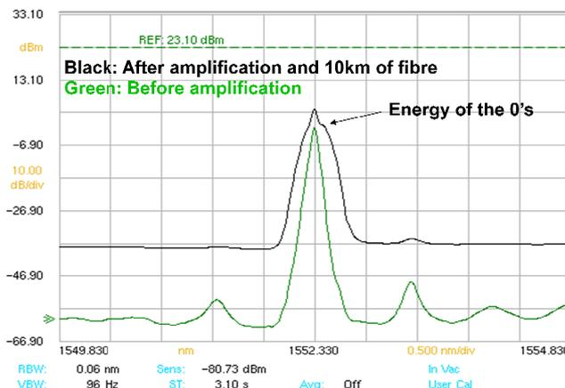
**Figure 3 Spectral Broadening caused by nonlinear effects in SOA saturation**
