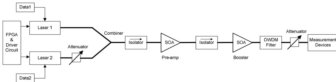
Figure 4 Burst equalisation system setup showing the two stage amplification
