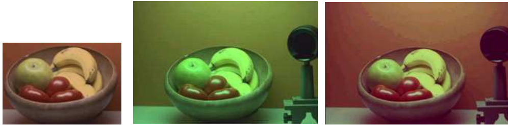
Figure 6: Cropped image A in Figure 2, Image B in Figure 2, and corrected version \mu_{AB} = (-33,38,-9) , error = 4.16%
