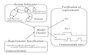
Figure 1. Model checking basic steps
