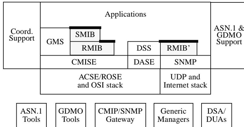
**Fig. 1. The OSIMIS Layered Architecture and Generic Applications**
