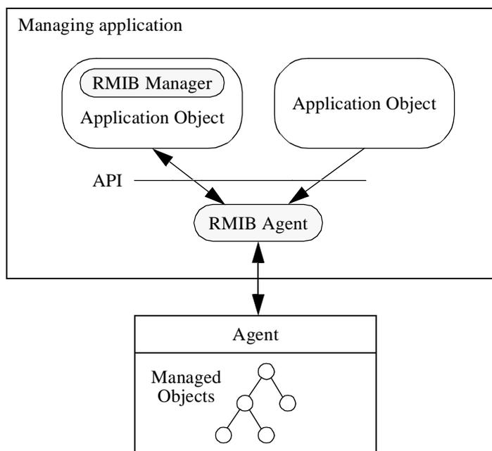
**Fig. 2. Remote MIB Model Interactions**
