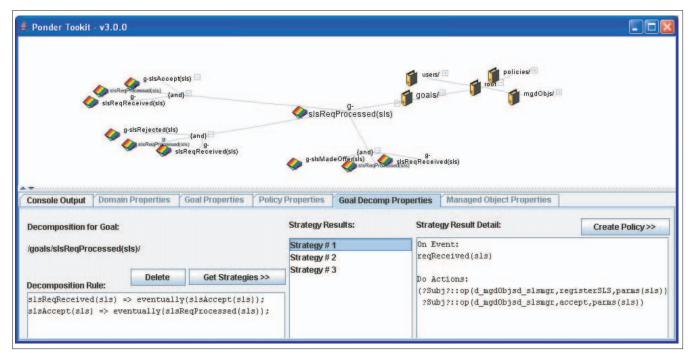
FIGURE 8. Policy refinement tool user interface. The top pane displays the domain hierarchy and the bottom pane has a number of detail tabs. Here we show the detail of a goal decomposition, together with the strategies derived. The decomposition rule (bottom left) describes the relationship between the sub-goals.
