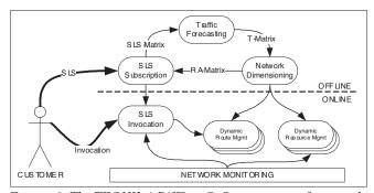
FIGURE 1. The TEQUILA DiffServ QoS management framework operates in an offline mode to determine the network configuration required to meet long term traffic needs; and an online mode that adapts to short-term variations.
