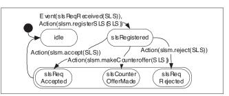
FIGURE 2. The Service Level Specification Subscription (SLS-S) module is responsible for handling new SLA subscription requests, deciding to accept, reject or make counteroffers based on the policies of the QoS management system.
