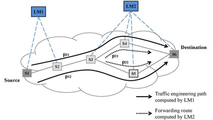
Fig. 7. Example of possible inconsistencies between routing decisions.
