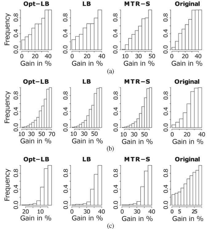
Fig. 13. Cumulative frequency graphs of the gain in terms of active line cards obtained by EM compared to the other schemes. (a) Abilene. (b) Geant. (c) Germany50.
