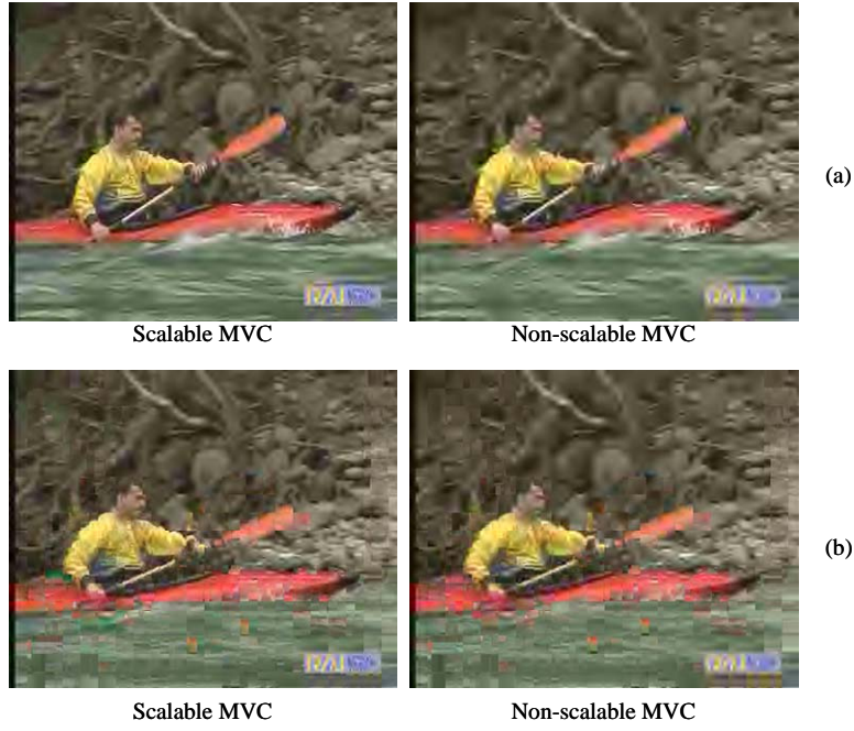
Figure 9: Comparison between scalable and non-scalable MVC employed in the codec of [6]: Visual comparison for the “Canoe”-sequence decoded at 256 kbps. (a) Frame 0. (b) Frame 2.
