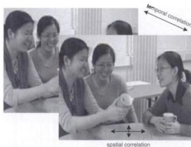
Figure 3: Temporal and Spatial correlation in two consecutive video frames; from "H.264 and MPEG-4 video compression: video coding for next-generation multimedia" [17]
