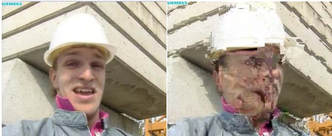
Figure 11: Distortion in the video at the client (right) as compared to the same frame in the encoded video at the server (left).
