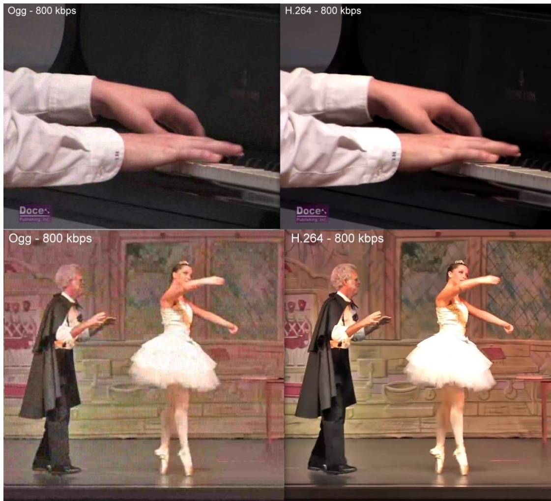
Figure 7: Two comparisons between OGG Theora encoded videos (left) and H.264/AVC encoded videos (right)
