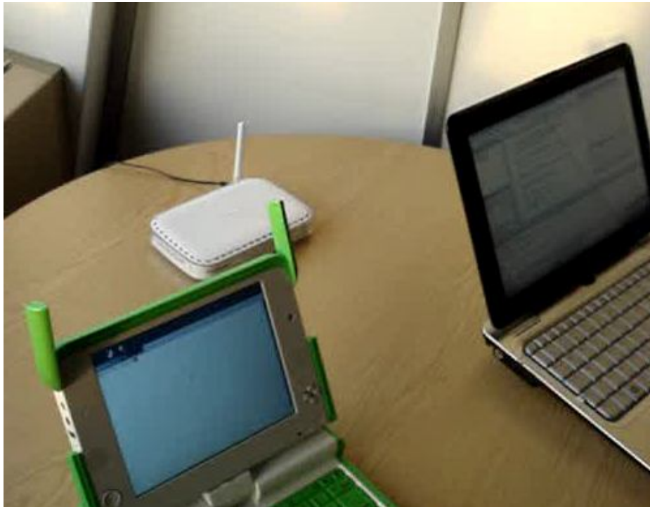
Figure 9: A picture showing the real hardware setup with the OLPC as the server, a HP laptop as the client and a netgear router.
