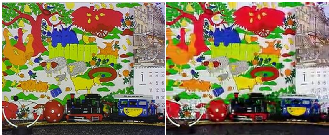
Figure 12: Artefacts in the video encoded with QP40 (right) as compared to the same frame in the original YUV video.
