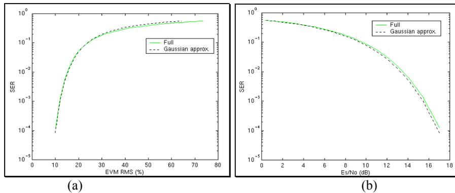
**Figure 4:** Symbol error rate results for 8-PSK with phase distortion when the phase has *Full* and Gaussian approximation PDFs versus: (a) EVM RMS; (b)  $E_s/N_0$ ,
