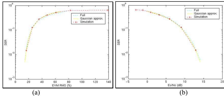
**Figure 5:** Symbol error rate results for 8-PSK with phase distortion when using analytical expressions (phase PDF employing *Full* and Gaussian approximation expressions) and computer simulations versus: (a) EVM RMS; (b) Es/No
