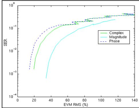
**Figure 2:** Symbol error rate versus EVM for 8-PSK system with complex (magnitude and phase), magnitude and phase distortion
