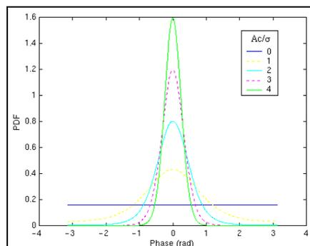
**Figure 3:** Phase PDFs for the PSK signal with bandpass Gaussian noise for  $A_c/\sigma$  ratios of 0, 1, ..., 4
