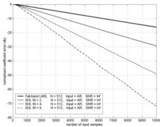
Fig.4 The NCEN for the proposed SIS against that of the Full-Band LMS for the AR input case.  $N(z) = 0$
