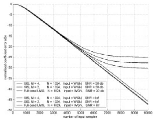
Fig.5 The NCEN for the proposed SIS against that of the Full-Band LMS when the input is a WGN process.
