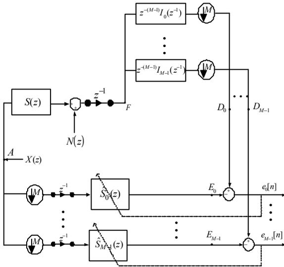
**Fig.2.** An equivalent representation of the SIS of Fig.1 with the decimators relocated and the matrix replaced by a FB.
