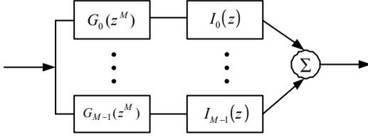
**Fig.3.** An arbitrary FIR system represented as the parallel interconnection of  $M$  systems each comprised by an interpolator and a sparse sub-filter.
