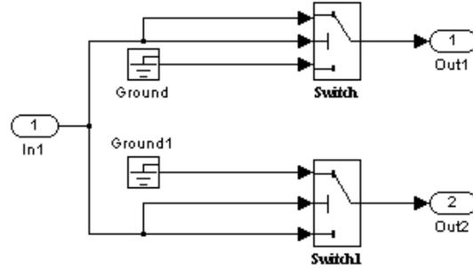
Figure 6. The block diagram for the switch subsystem.
