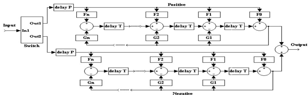
Figure1. Non-linear System Model.
