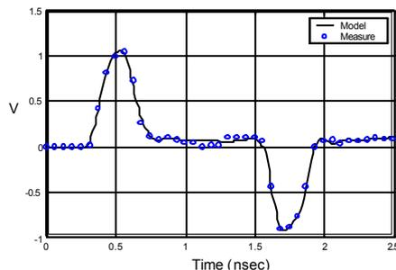
Figure 9. The o/p from the model when the i/p two pulses.
