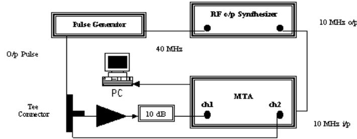
Figure 2. Time domain scattering function measurement system for amplifier.
