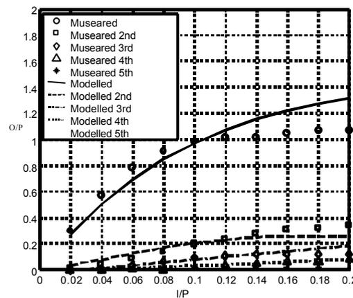
Figure 13. Input-output characteristics of the non-linear amplifier.
