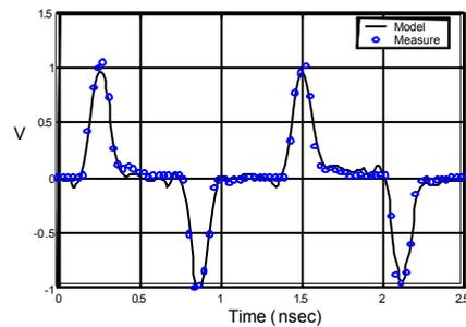
Figure 10. The o/p from the model when the i/p four pulses.
