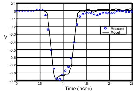
Figure 8. Negative pulse responses of the amplifier model.
