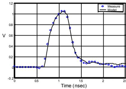
Figure 7. Positive pulse responses of the amplifier model.
