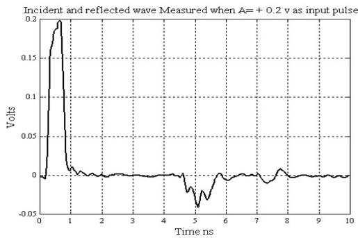
Figure 3. Measured incident and reflected waveforms.
