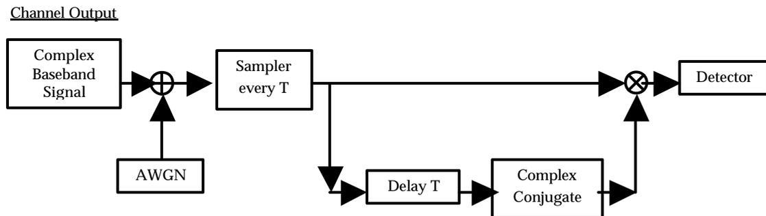
Figure 3: The Block diagram of the channel, noise and receiver.
