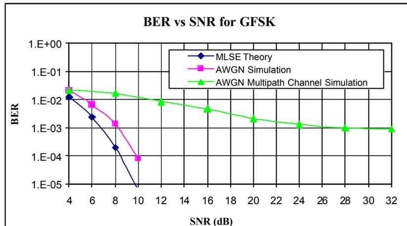
Figure 4: Average BER performance of the system under AWGN and multipath fading channel.
