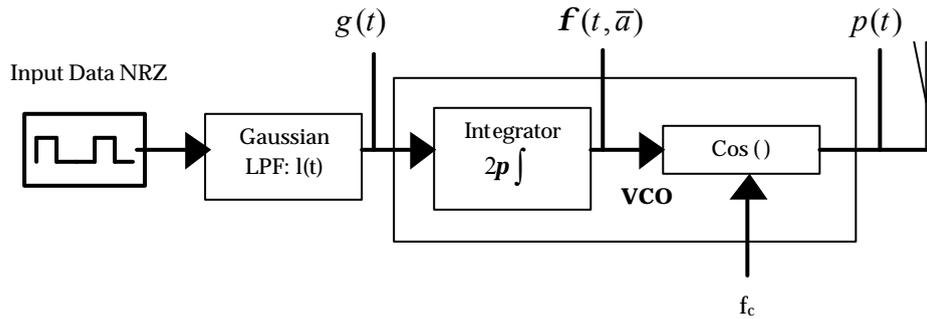
Figure 1: The block diagram of the GFSK transmitter.
