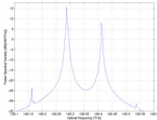
**Figure 3: Optical spectrum for spacing of 1 nm.**
