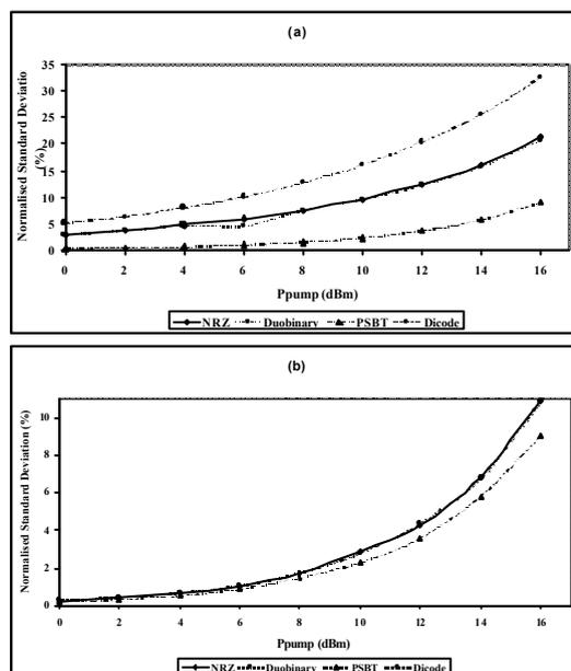
Figure 2: XPM as function of pump average power.
