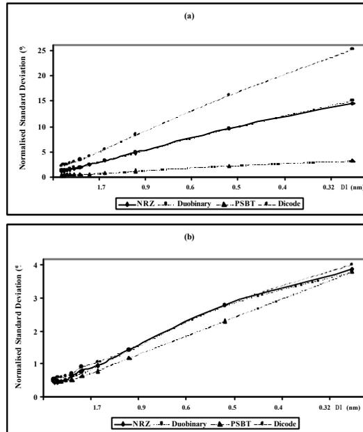
Figure 1: XPM as function of wavelength separation with pump power of 10 dBm (note the  $1/D\lambda$  scaling of the horizontal axis).
