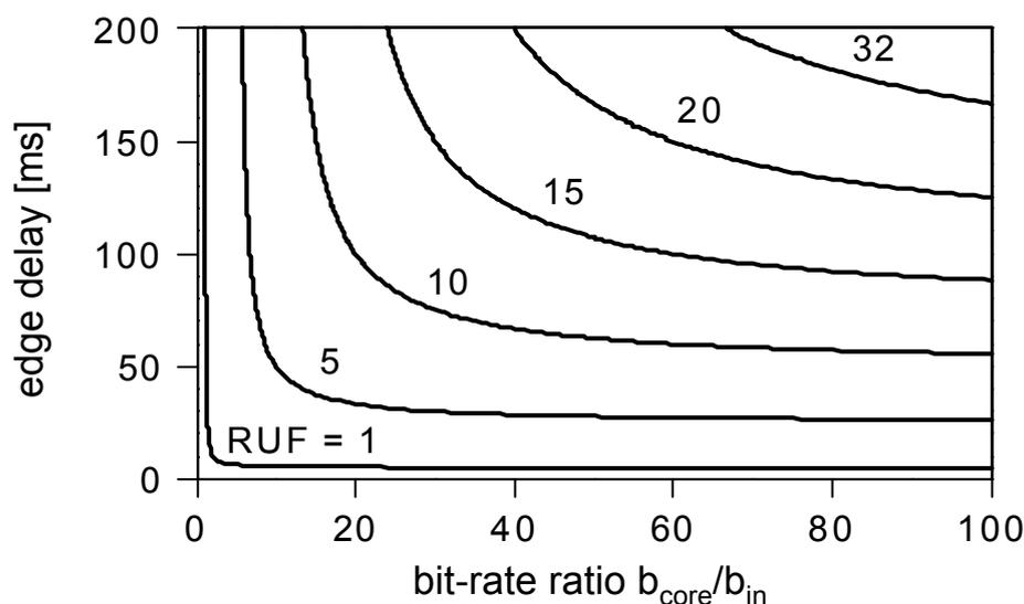
**Fig. 3. Wavelength re-use factor (RUF) as a function of edge delay,  $t_{edge}$  and bit-rate ratio  $A$  for round-trip time  $t_{RTT} = 5 \text{ ms}$**
