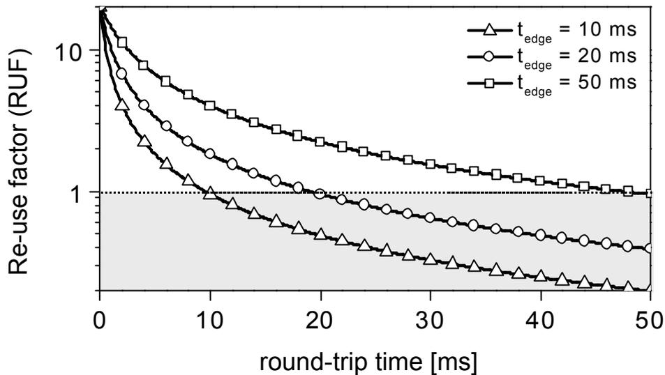
**Fig. 4. Re-use factor  $RUF$  as a function of the round-trip time ( $t_{RTT}$ ) for  $t_{edge} = 10, 20, 50$  ms and bit-rate ratio  $A = 20$ . Shaded region: network requires more wavelengths than static WRON**
