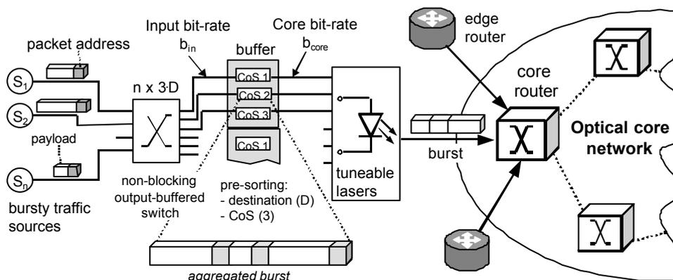
**Fig. 1. Model of electronic edge routers for burst aggregation, connected to the high-speed DWDM optical core network**
