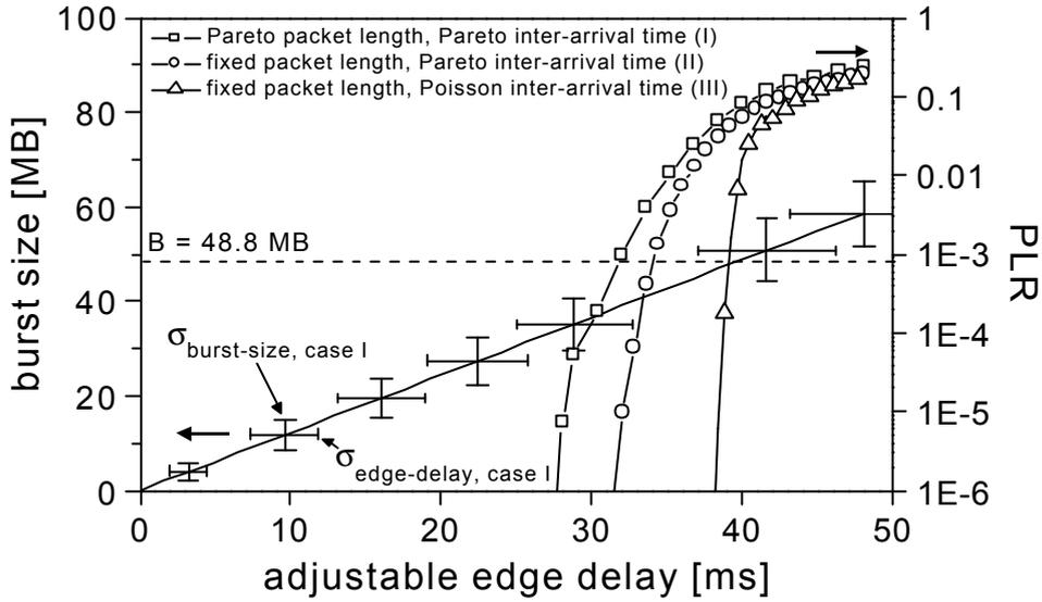
**Fig. 2. Burst size, edge delay distribution and resulting PLR for three different traffic statistics**
