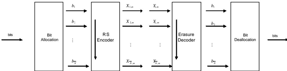
Figure 3. Coded DMT transmitter
