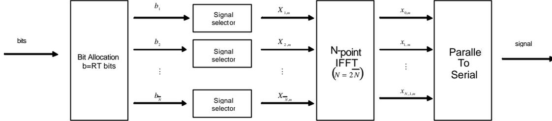
Figure 1. Baseline DMT transmitter
