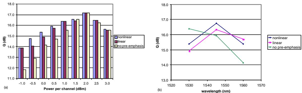
Figure 3. (a) Worst channel Q-values for the 35x84km span link with RZ modulation showing results obtained from full nonlinear simulations using the optimum pre-emphasis predicted by full nonlinear simulations, linear simulations and with no pre-emphasis. (b) example spectrum, showing Q-values from full nonlinear simulations using the optimum pre-emphasis predicted by full nonlinear simulations, linear simulations and with no pre-emphasis at 0dBm per channel
