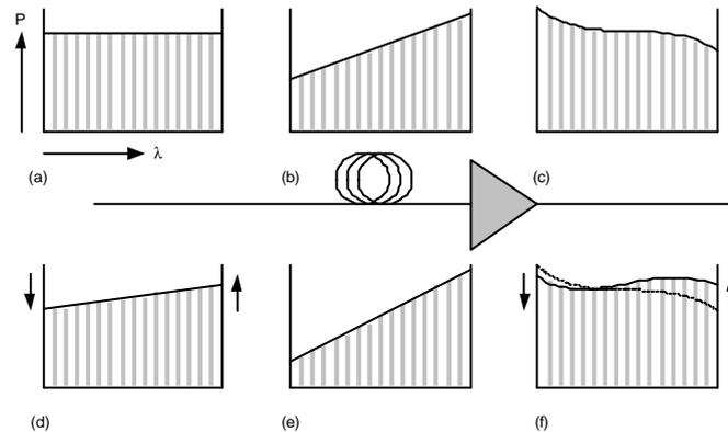
Figure 1. An illustration of the principle of input channel power pre-emphasis. Figs. (a), (b) and (c) show the evolution of a WDM signal through an optical fibre span and an EDFA using no pre-emphasis. Figs. (d), (e) and (f) show the same evolution but with pre-emphasis to equalise the net gain at the end of the transmission link.
