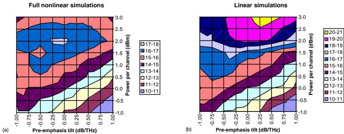
Figure 2. Q-value contour map for 35x84km span link using per span dispersion compensation for (a) full nonlinear simulations (b) linear simulations
