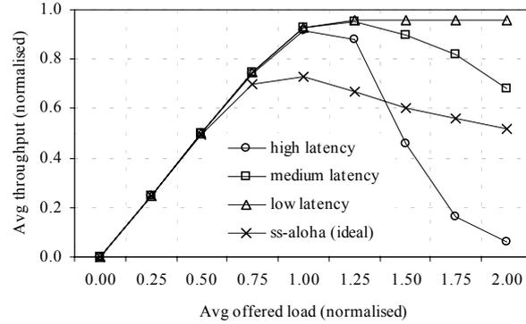
Fig. 2 Throughput versus offered load in OSSS+RED and ideal SS-ALOHA
