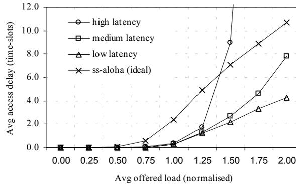
Fig. 3 Average access delay versus offered load in OSSS+RED and ideal SS-ALOHA
