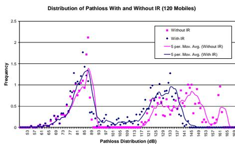
Figure 5: Comparison of Pathloss Distribution With and Without IR (120 MSs)
