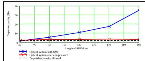
Fig. 7. Dispersion penalty of optical communication system.
