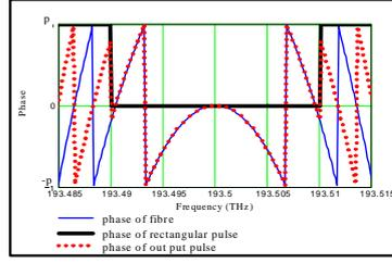
Fig. 2. The phases of SMF, rectangular and output pulse.
