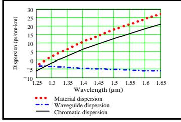
Fig. 1. Variation of MD, WD and CD due to wavelength.
