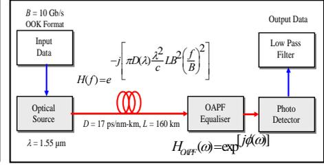
Fig. 3. Optical Communication System using SMF.
