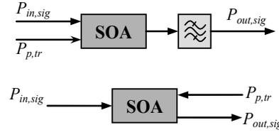
Fig. 3. Assist light injection set-up in co and counter propagative configurations.
