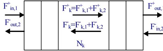
Fig 2. Schematic diagram of the SOA, longitudinally divided into sections.
