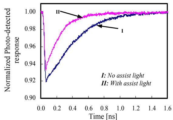
Fig. 7. Normalized measured gain recovery photo-detected response.
