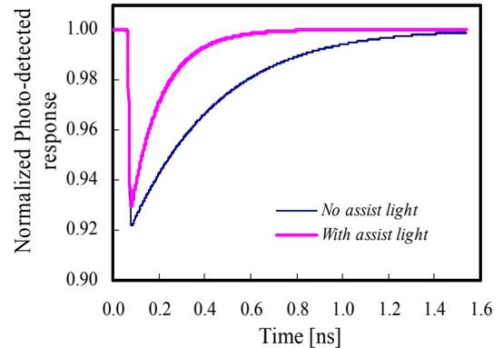
Fig. 5. Normalized calculated gain recovery photo-detected response.
