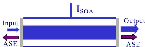
Fig. 1: SOA schematic diagram.
