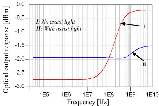
Fig. 4. Simulation results of optical output signal frequency responses in absence and in presence of an assist-light.
