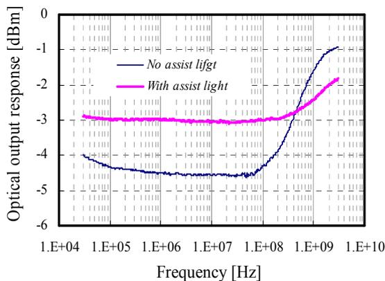
Fig. 6. Optical output signal frequency responses in absence and in presence of an assist-light.
