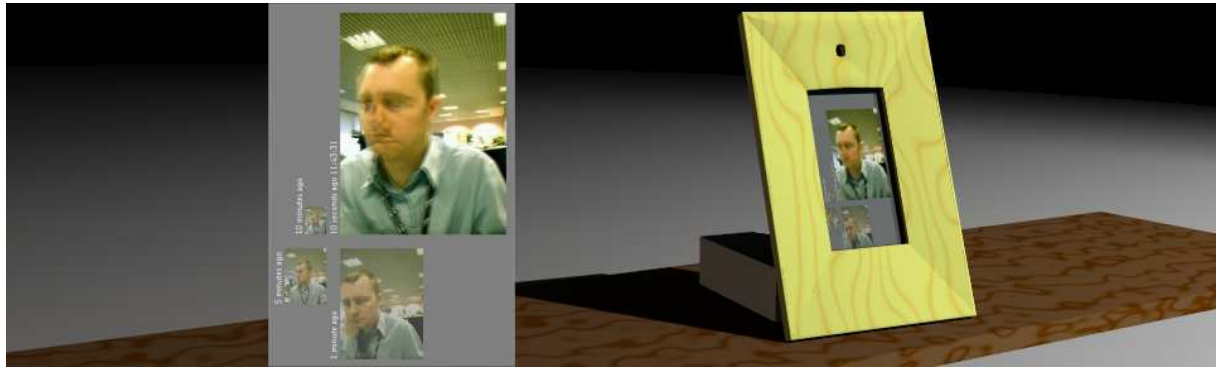
Figure 1: Model of a ‘smart’ picture frame displaying Video Snapshots. Overlaid, spiral history of previous snapshots, largest image is most recent - 10 seconds ago, 1 minute ago, 5 minutes ago, 10 minutes ago.
