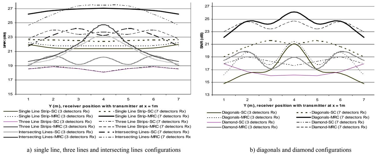
Figure 4: Signal-to-noise ratio (SNR) distribution for five different spot diffusing patterns under three and seven detectors angle diversity receivers with SC and MRC (along room width)
