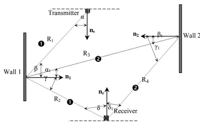
Figure 2: Ray tracing for first and second reflections
