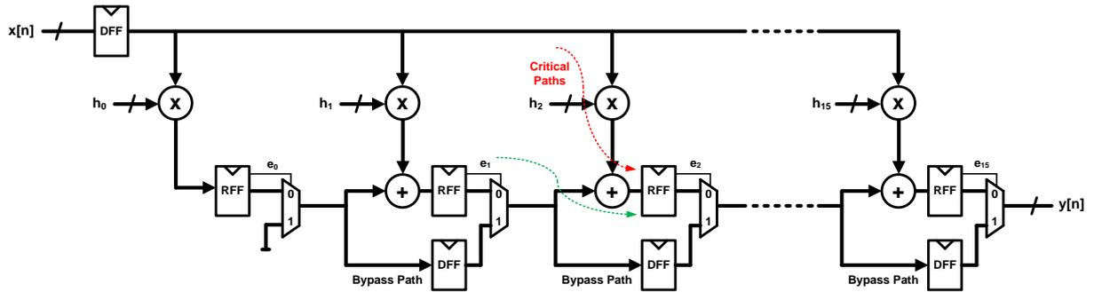
Figure 1: Proposed filter structure with error mitigation
