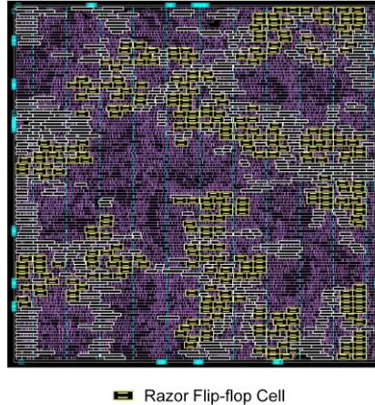
Figure 2: Layout of the Robust FIR Filter
