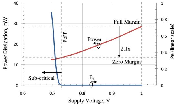
Figure 3: Simulation of Power Dissipation and  $P_e$  vs.  $V_{dd}$
