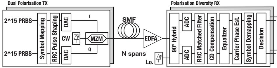
Figure 1: Simulation system diagram for SC-PDM-QPSK.
