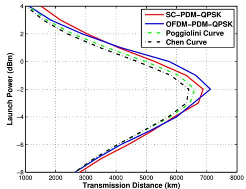
Figure 4: Launch power vs. transmission distance for 9 WDM 28GBaud channels at a channel spacing of 28.875GHz, BER of  $4 \times 10^{-3}$  (FEC limit)
