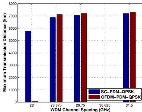
Figure 3: Maximum transmission distance -2dBm per channel, for different channel spacing, BER of  $4 \times 10^{-3}$  (FEC limit)
