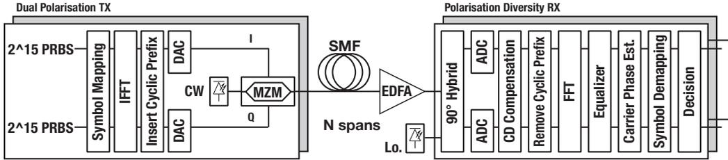
Figure 2: Simulation system diagram for OFDM-PDM-QPSK.
