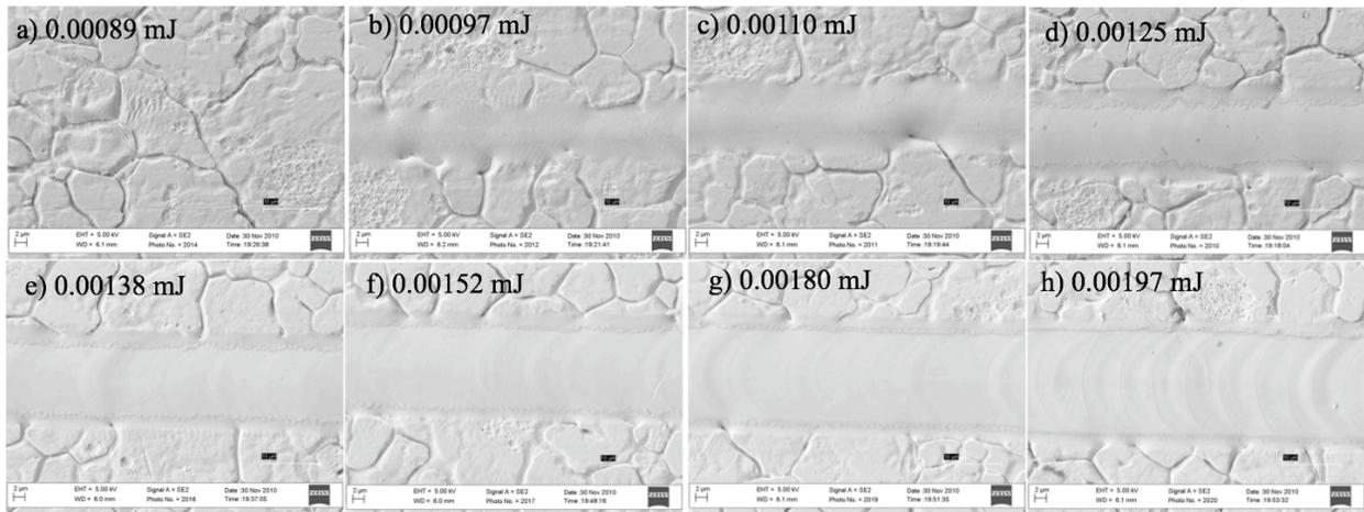
Figure 3: Shows SEM (Zeiss™ 1640 crossbeam) images of material responses of SS 304 stainless steel using 100 ps pulses with a range of pulse energies of  $E_{\text{pulse}} = 0.89 \mu\text{J} - 1.97 \mu\text{J}$ .
