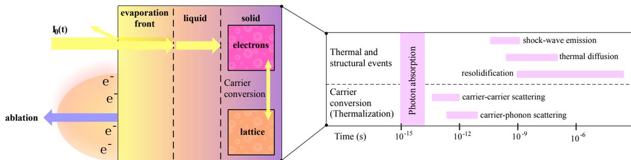
Figure 1: Timescales and the physical mechanisms associated with picosecond pulse interaction with matter.
