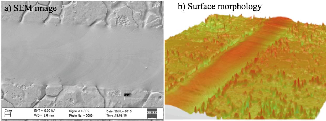
Figure 4: a) Shows SEM image of SS 304 stainless steel using 100 ps pulses with a pulse energy of  $E_{\text{pulse}} = 2.08 \mu\text{J}$  and b) the surface morphology (Veeco™ NT3300 white light interferometer).
