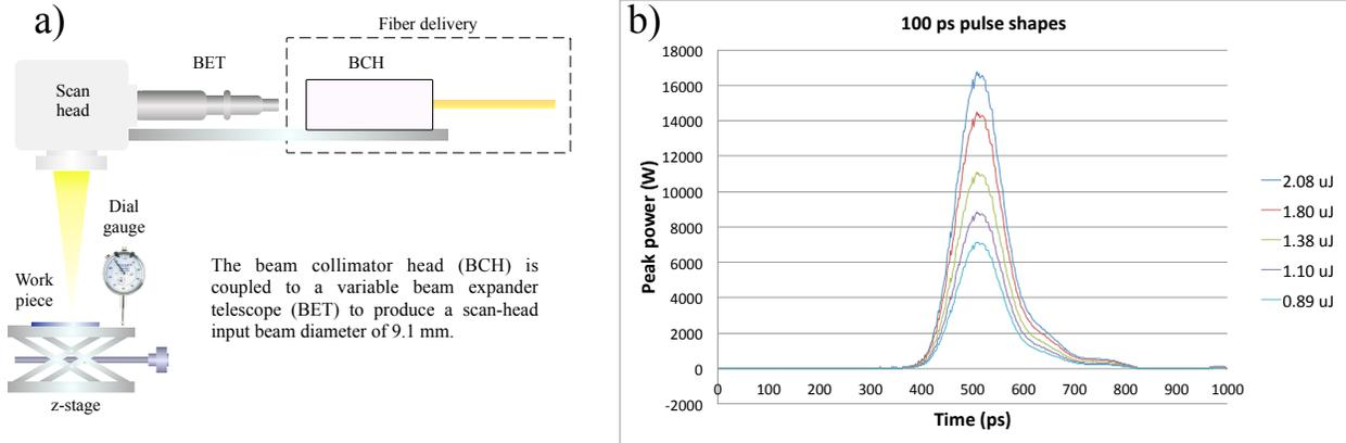
Figure 2: a) The test rig and b) the pulse shapes and peak powers for a range of pulse energies from  $E_{pulse} = 0.89 \mu J - 2.08 \mu J$ .
