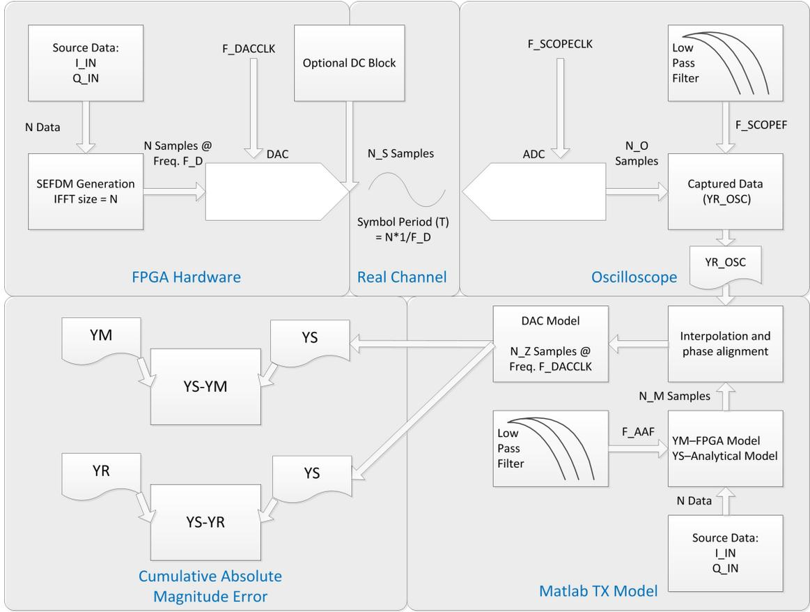
Figure 1: Verification methodology block diagram
