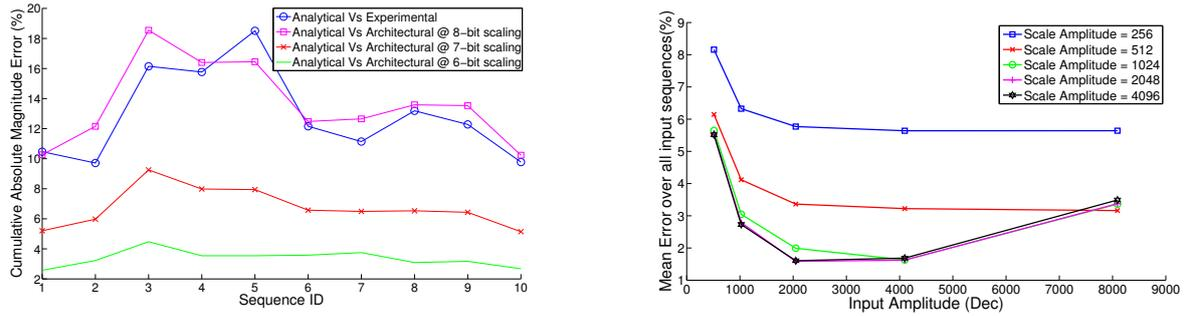
Figure 2: Cumulative absolute magnitude error for experimental and architectural signals with different bit scaling against analytical signals (left) and error performance with different internal and external data amplitudes (right)
