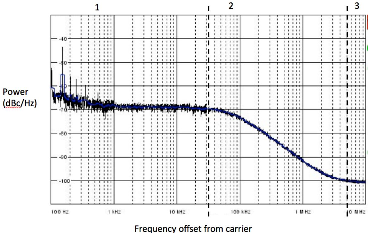
Figure 2 - Showing the single side band phase noise of the device mode locked with 15dBm from the Synthesiser, and at a drive current of 172mA
