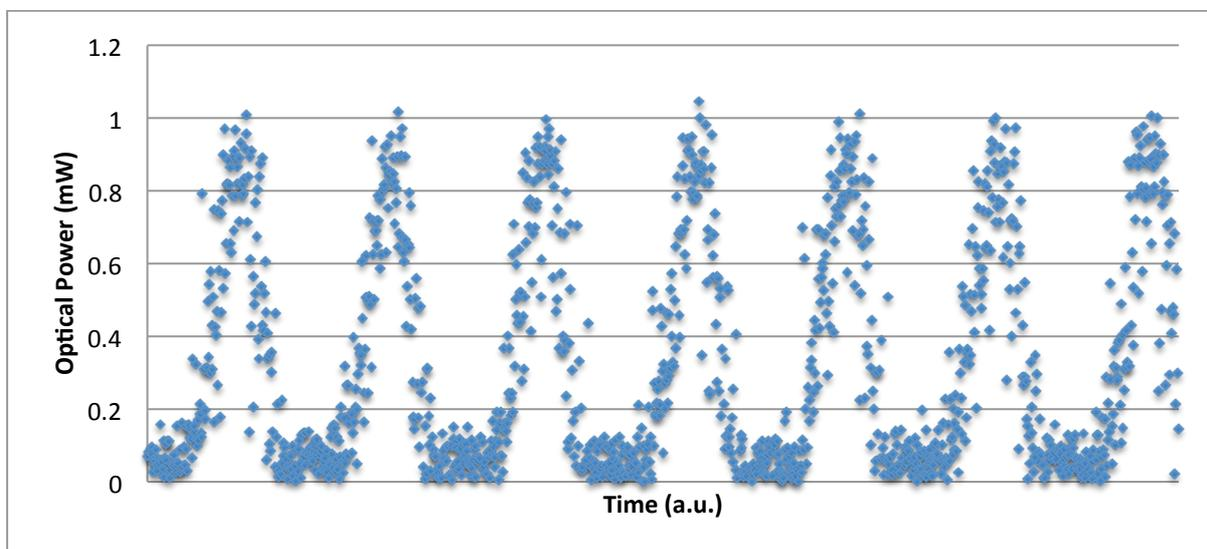
**Figure 3 Shows the optical pulse as shown on the sampling oscilloscope, after the pulses have passed through a 1nm optical filter**
