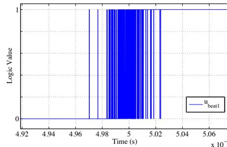
Figure 4 – Glitch on the output clock
