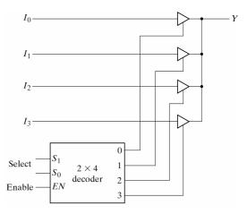
The use of a decoder ensures that no more than one buffer control input is active at any given time.
