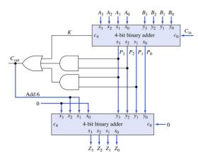
Whenever  $C_{out} = 0$ , the outputs from the upper 4-bit binary adder are sent to the lower 4-bit adder and decimal 0 is added.
