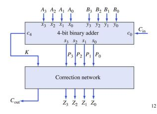
Since each operand digit does not exceed 9, the output sum cannot be greater than 9 + 9 + 1 = 19, the 1 in the sum being an input carry.
