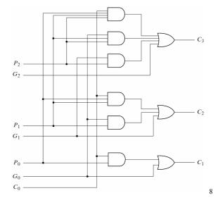
The construction of a 4-bit adder with a carry lookahead scheme is shown below:
