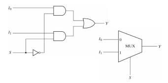
The circuit has two data input lines,  $I_1$  and  $I_2$ , one output line *Y*, and one selection line *S*.
