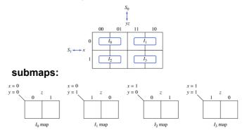
Grouping the 1-cells, the expressions for the subfunctions may be written. That is,  $I_0 = z'$ ,  $I_1 = 1$ ,  $I_2 = z$ , and  $I_3 = 0$ . The logic realization is as before.
