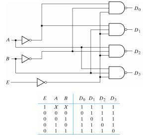
A decoder with enable input can function as a *demultiplexer*. The above decoder can function as a 4-to-1-line demultiplexer when *E* is taken as a data input line and *A* and *B* are taken as the selection inputs.
