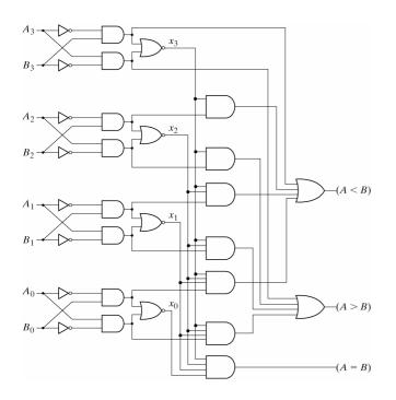
The four *x* outputs are generated with X-NOR circuits and applied to an AND gate to give the output binary variable (A = B).
