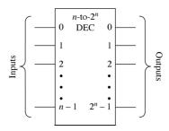
The structure of a such decoder is straightforward. Consider the truth table of a 3-to-8-line decoder:
