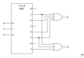
The *n*-to- $2^n$ -line decoder is only one of several types of decoders. *Function-specific* decoders exist having fewer than  $2^n$  outputs. Examples include the BCD-to-decimal decoder (7442A) and the BCD-to-7-segment decoder.
