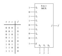
The realization is obtained by placing x, y, and z on the  $S_2$ ,  $S_1$ , and  $S_0$  lines respectively, logic-1 on data input lines  $I_0$ ,  $I_2$ ,  $I_3$ , and  $I_5$  and logic-0 on the remaining data input lines. Also the multiplexer must be enabled by setting E = 1.
