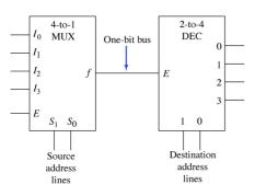
By using *n* of the structures shown above in parallel, an *n*-bit word from any of four source locations is transferred to the four destination locations.
