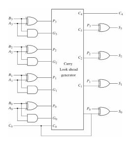
All output carries are generated after a delay through two levels of gates. Thus outputs  $S_1$  through  $S_3$  have equal propagation times.
