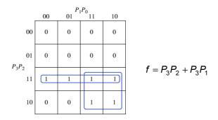
The condition for a correction and an output carry can be expressed by the Boolean function:
