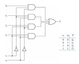
A multiplexer is also called a *data selector*, since it selects one of many inputs and steers the binary information to the output line.
