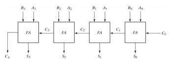
An *n*-bit adder requires *n* full adders with each output carry connected to the input carry of the next higher-order full adder.
