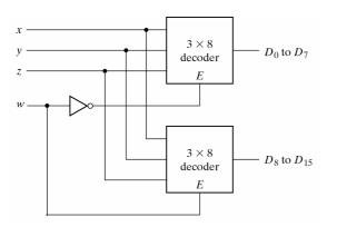
When w = 0, the top decoder is enabled and the other is disabled. The bottom decoder outputs are all 0's, and the top eight outputs generate minterms 0000 to 0111.
