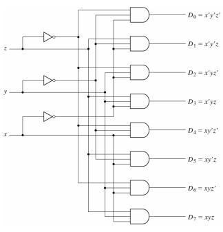
A particular application for this decoder is binaryto-octal conversion. The input variables represent a binary number, and the outputs represent the eight digits in the octal number system.
