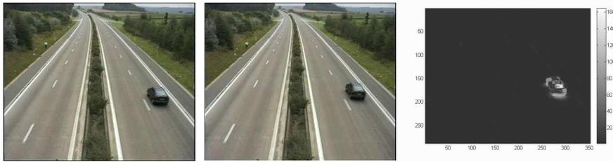
**Fig. 2.** Two adjacent frames and their intensity difference
