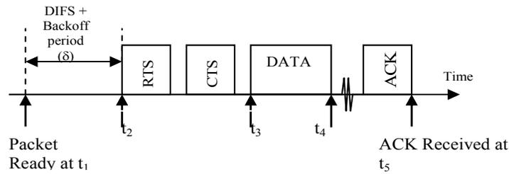
Fig. 1. IEEE 802.11 unicast packet transmission sequence
