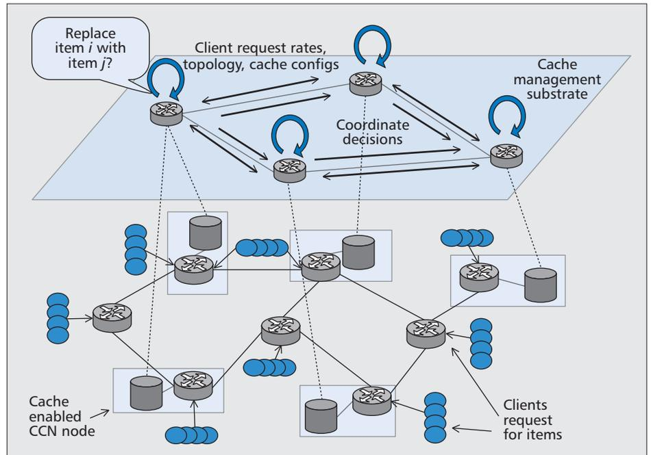
Figure 6. Cache management substrate in content-centric networks.
