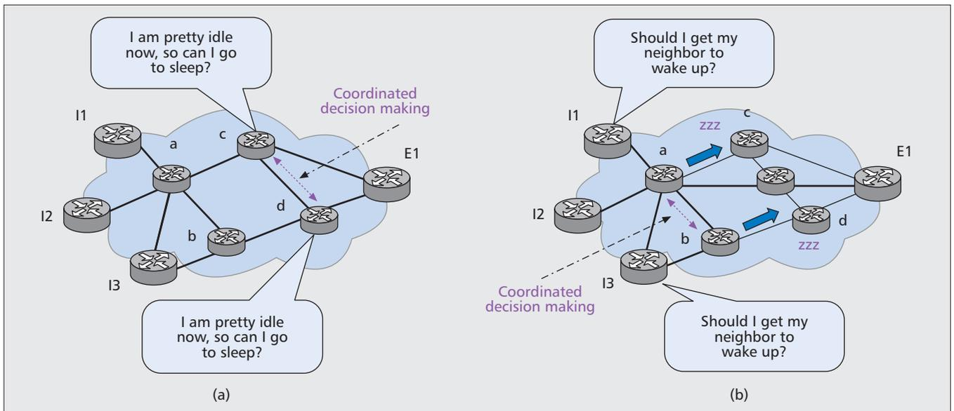
Figure 5. Two types of router-level coordination.
