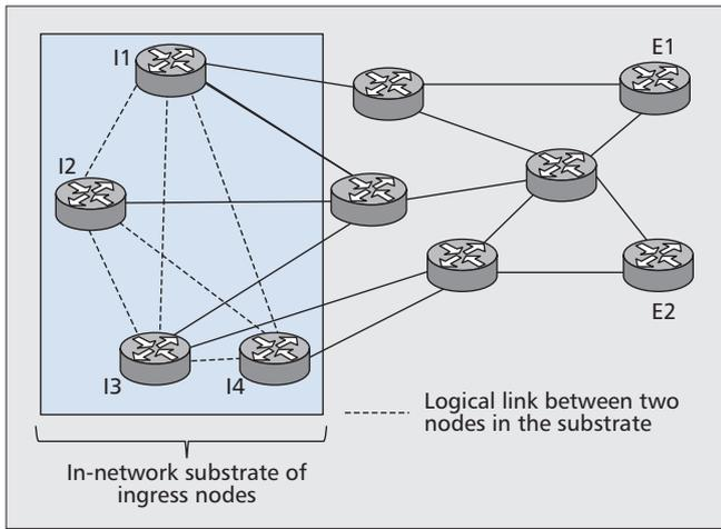
Figure 4. Example of a network and its associated full-mesh in-network substrate of ingress nodes.
