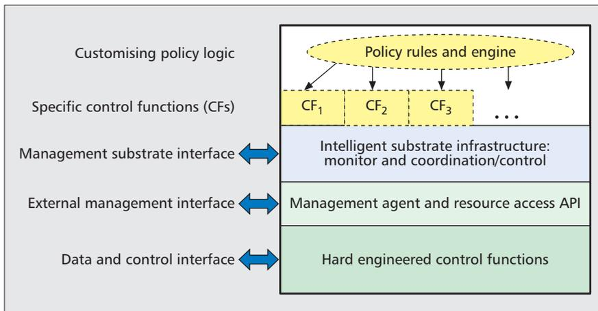
Figure 2. *Self-managed node architecture.*
