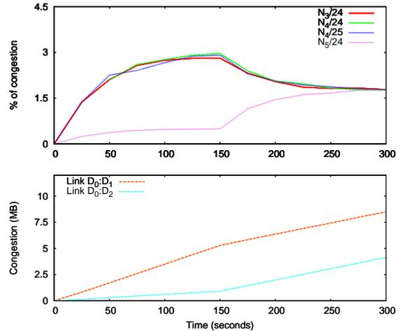
Figure 2: Upstream congestion estimate and congestion volume viewed from  $D_0$ . At  $t = 150s$ ,  $D_0$  switches path for destination  $N_4/25$  and through  $D_2$ .
