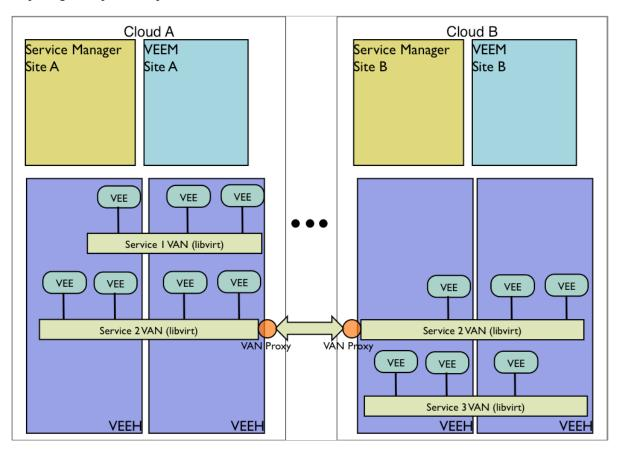
Figure 2: VANs and services running on two RESERVOIR sites
